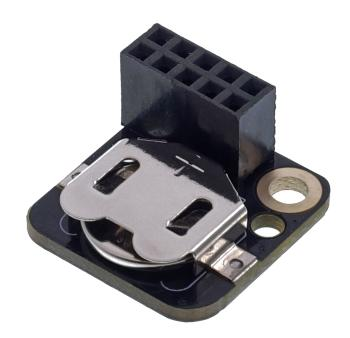
The DS3231 system is a complete RTC clock, which is distinguished by high precision in time measurement. Excellent
