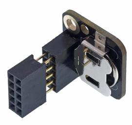
In this configuration, the KAmodRPI RTC module is placed above the radiator and the entire set can operate properly.
